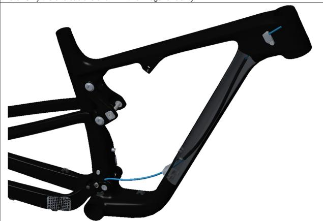
Pour isopropyl alcohol down Foam Tube to lubricate foam tube.
