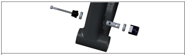
1) Use a blind puller seated against the bearing inner races to remove main pivot bearings.
