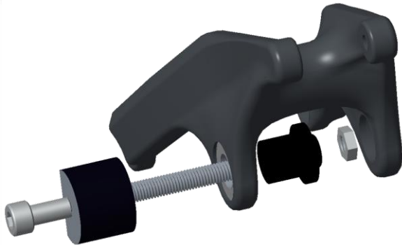
Chain Stay Bearing Removal (DR11197 Tool)
